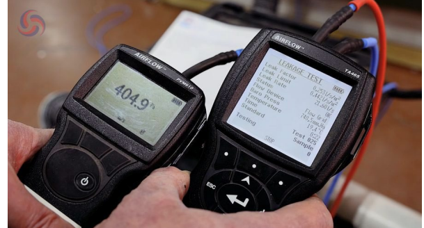
Figure 10. Pressure gauge stabilised at -404.9 Pa (close to the -400 Pa negative test target) with leakage tester reading alongside.
