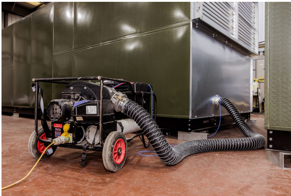
Figure 4. Calibrated leakage tester (e.g., PANDA model)
