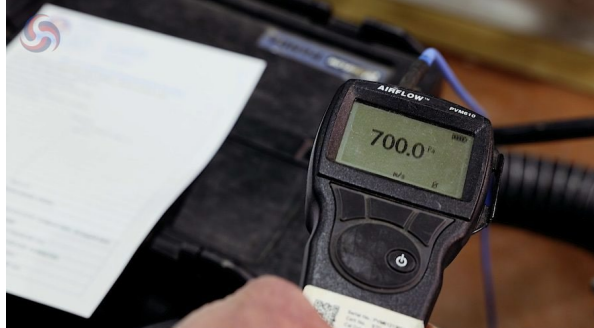
Figure 9. Calibrated digital pressure gauge showing 700.0 — required positive test pressure achieved.
