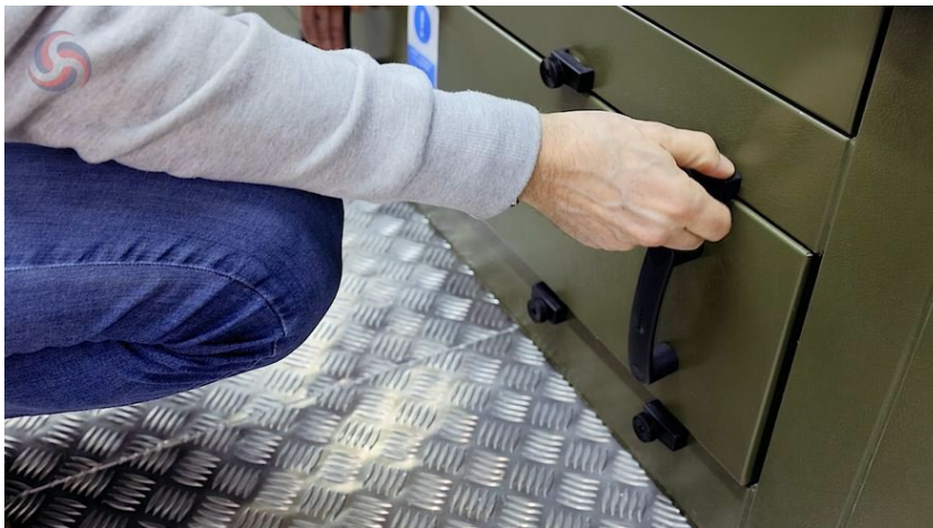
Figure 9. Refitted tray with handle accessible — confirm the tray sits square and level against the rear stop.
