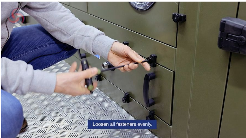
Figure 5. Loosening all retaining-panel fixings evenly before withdrawing the panel.
