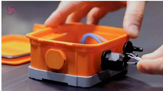
Figure 10. Sensor housing opened ready for termination — verify terminal identification before insertion.
