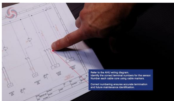
Figure 5. Referring to the AHU wiring diagram to identify the correct terminal numbers for the sensor.
