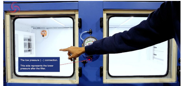
Figure 14. Low pressure (-) tube connection between the two filter doors - this side represents the lower pressure after the filter.
