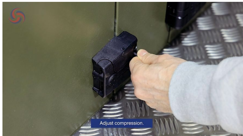
Figure 11. Adjusting the compression on the latch cam incrementally before re-checking the seal.
