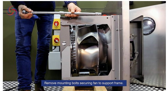
Figure 14. Removing the mounting bolts securing the fan to the support frame.
