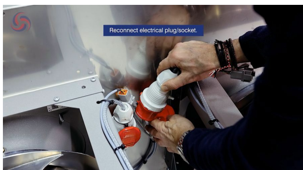
Figure 20. Reconnecting the electrical plug/socket. Ensure the cable routing follows the original path.
