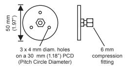
Universal Fitting Kit for immersion sensor use in existing pockets (ACC/UF)
