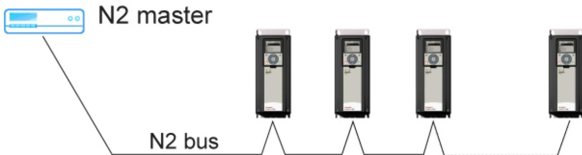
Figure 4. Principal example diagram of Metasys N2
