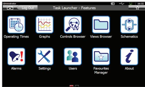
The IQVIEW8 user interface can, **and should**, be configured to present end users with only the functionality they need, with any irrelevant features or information hidden from view.
