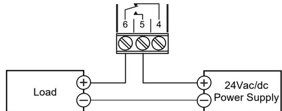
Load on when alarm not present (relay de-activated)
