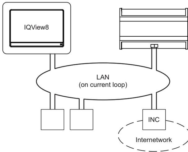
In order to join an internetnetwork, an INC type device (e.g. IQ4NC) will be required elsewhere on the current loop LAN.
