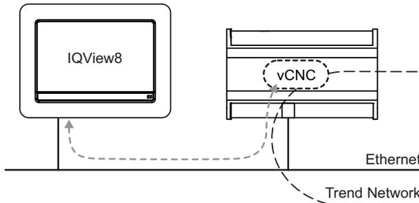
The IQVIEW8 supports either static or dynamic (DHCP) IP addressing. DHCP is enabled by default.
