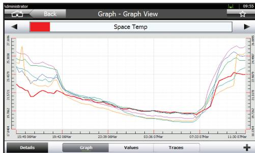
It is possible to zoom in on selected parts of the graph so that it can be seen in more detail, display spot values or to view the underlying data from the graph.
