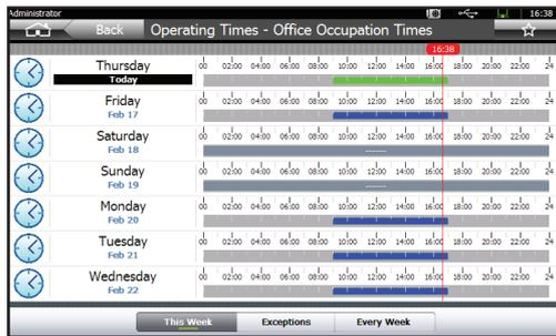
The system date, time and daylight saving dates can also be configured using IQVIEW8.
