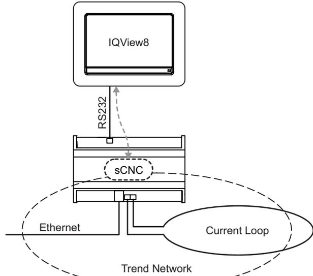
The supervisor port (sCNC) must be configured to allow network access to the Trend network.
