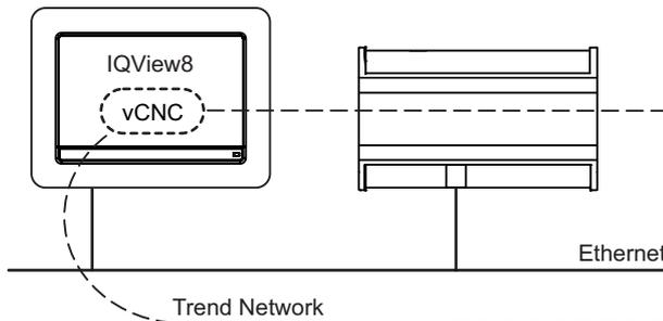
When connecting using a vCNC in another device IQVIEW8 takes the network address of that vCNC. Alarms sent to the vCNC will be received by the IQVIEW8.
