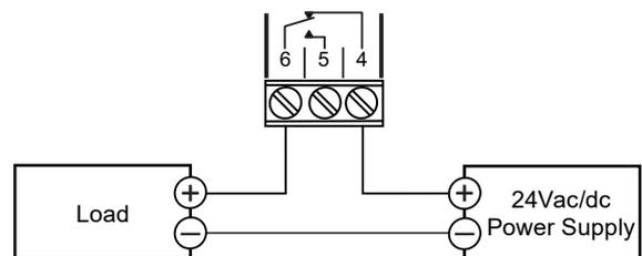
**Caution:** The relay contacts **must not** be used to switch to mains voltage; see page 11 for details of contact ratings.
