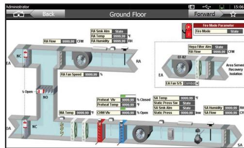
Schematic pages are typically displayed full screen, i.e. without any navigational features of the standard interface being visible; navigation between Schematic pages can be provided by buttons/controls built-in to the pages. Schematics are created using Trend's 963 Supervisor and exported for use with IQVIEW8 using the 963 Schematic Export Utility. See the 963 Schematic Export Utility Manual (TE201242) for details.
