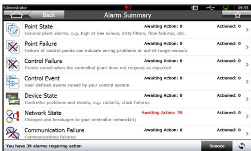
Unactioned alarms can be viewed, and actioned, or snoozed from the Unactioned Alarms Screen.
