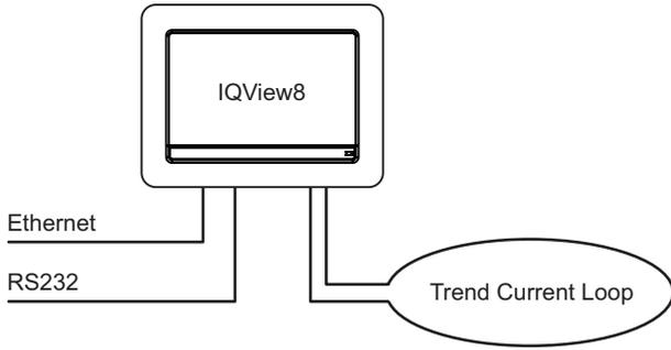
The IQVIEW8 is not designed for multi-site operation, although more than one IQVIEW8 can be connected to the same site. It cannot access autodialed sites (e.g using a TMN), and it cannot receive alarms from sites using autodialing or TCP/IP dial up.
