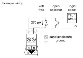
The volt free contact has a nominal wetting current of 270  $\mu A.$  The input is ON when the contact is closed.
