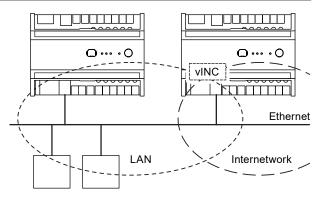
In addition, the IQ422 has the ability to join an internetwork using its virtual INC (see 'Networking' on page 4 for further details).
