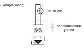
**Digital input:** Used for a volt free contact, logic circuit (e.g. TTL, CMOS), open collector (transistor) or open drain (FET).
