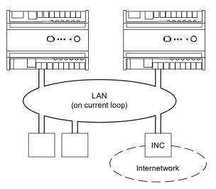
Note: In this configuration IQ422 cannot join a Trend LAN on Ethernet. However, access by IP is still possible.
