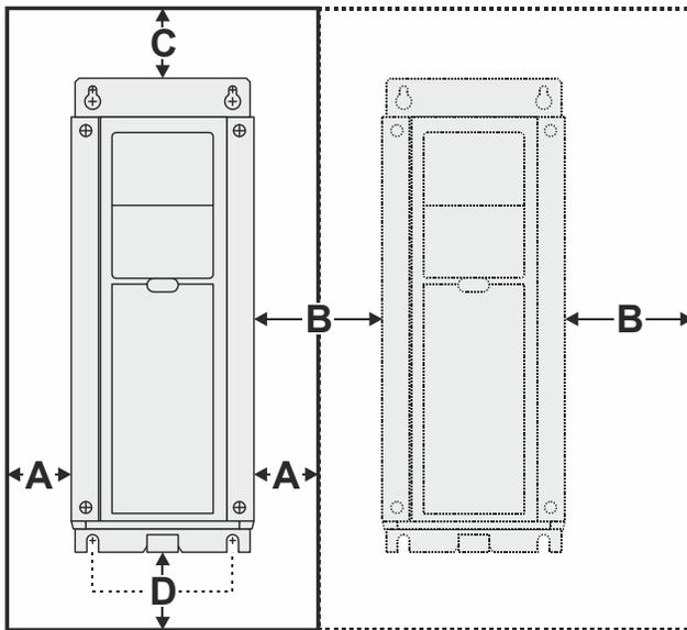
Fig. 4. Distances to ensure proper cooling
