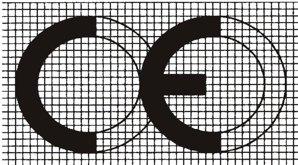
The CE marking must have a height of at least 5 mm. If the CE marking is reduced or enlarged the proportions given in the above graduated drawing must be respected.
